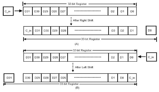
Fig. 7.A. 32-bit Right Shift Operation, 7.B. 32-bit Left Shift Operation.
