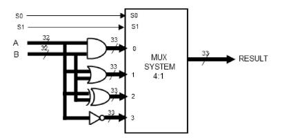
Fig. 7. 32-bit Logic Unit
