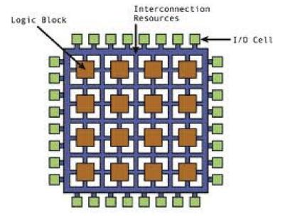
Fig. 4. FPGA Structure
