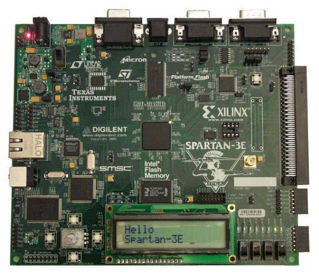
Fig. 3. Spartan-3E FPGA Starter Kit Board
