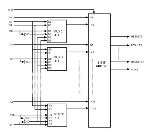
Fig. 6. 32-bit Arithmetic Unit
