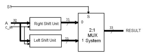
Fig. 8. 32-bit Shifter Unit
