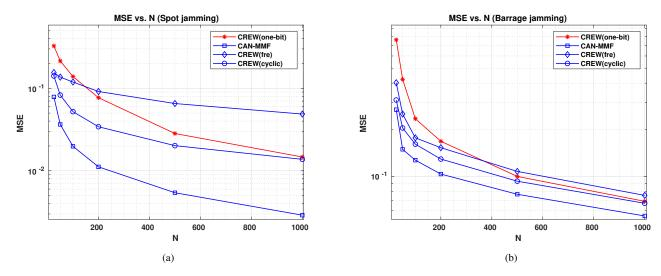
Fig. 1. MSE values obtained by the different design algorithms for (a) spot jamming with normalized frequency  $f_0 = 0.2$ , and (b) barrage jamming in the normalized frequency interval  $[f_1, f_2] = [0.2, 0.3]$  for the unimodularity constraint on the transmit sequence.
